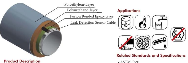
This invotive Thermal Insulation coating enables monitoring and detectionn of Leaks before damages occur. Leak Detection Sensor Cable embedded in the Polyurethane foam after the anti-corrosion layer of fusion Bonded Epoxy based followed by high density polyethylene casing that keeps any leakage trapped inside is designed for great insulation protection.
